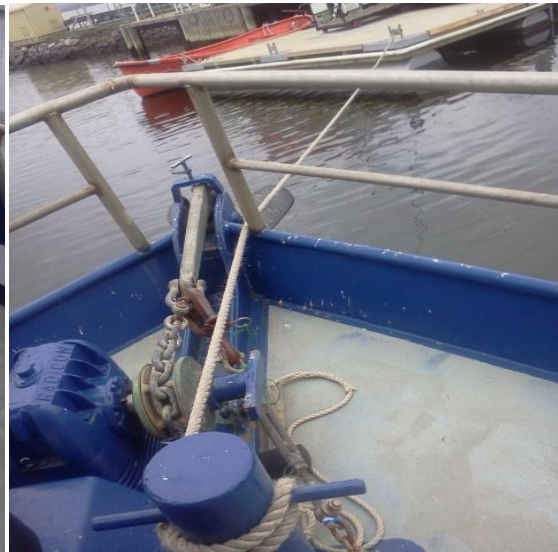
Figure 2 Bow mooring arrangement
